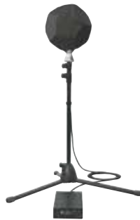
Miniature dodecahedron speaker for room acoustic measurements
